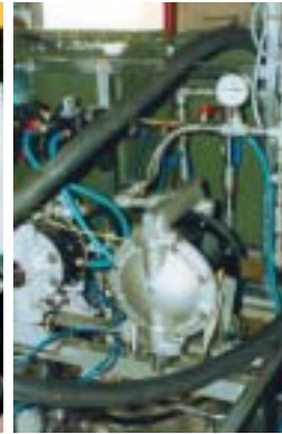
ARO diaphragm pumps used in chemical laboratory.
