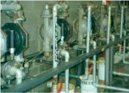
Bank of PD20A-BSS-STT used for solvent manufacturing.
