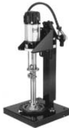
Single post ram - for extrusion of up to 500.000 cPs material. 360° rotation allows to serve three 200 l containers.
