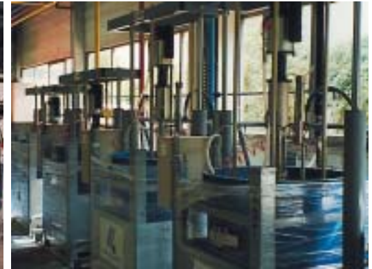
Special extrusion pump packages for sheet fed inks used for high volume consumption.
